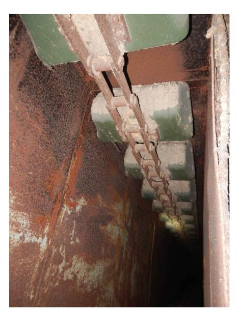
**K**4 INTERIOR DETAIL OF THE GRAIN ELEVATOR SHOWING THE CONTAINERS AND CONVEYOR SYSTEM TO BE DISPLAYED THRU THE EXISTING HATCH DOORS.
