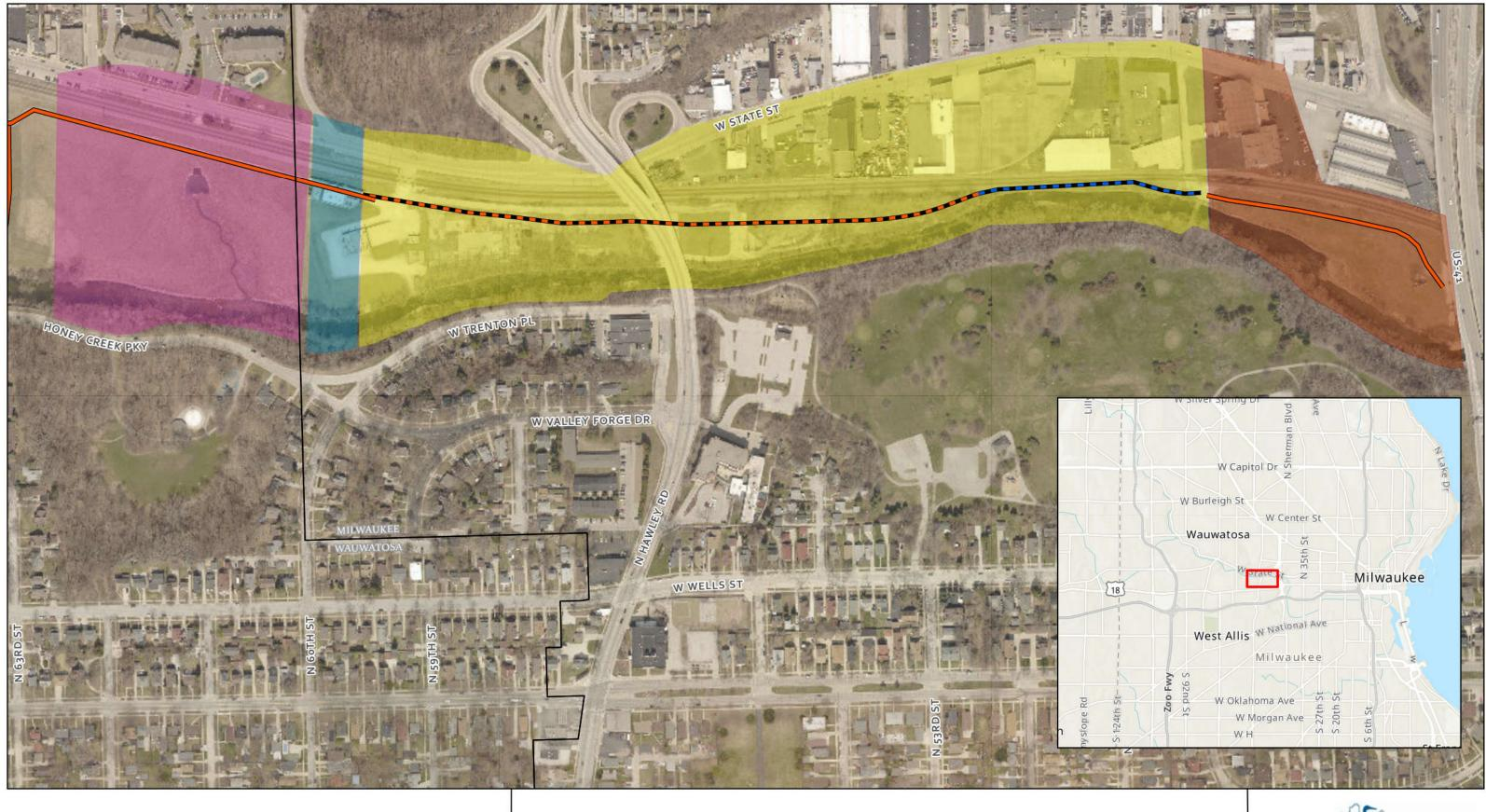
Phase 2A Existing Earthen Levee 59th and State Pump Station ---- Proposed Floodwall Phase 2B --- Proposed Earthen Levee Phase 1
