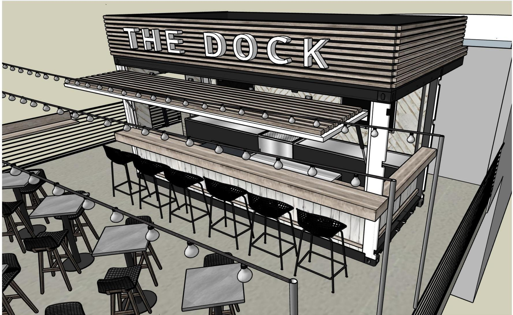
East and west sides of the bar structure shall have this same horizontal wood detailing as the north side.
