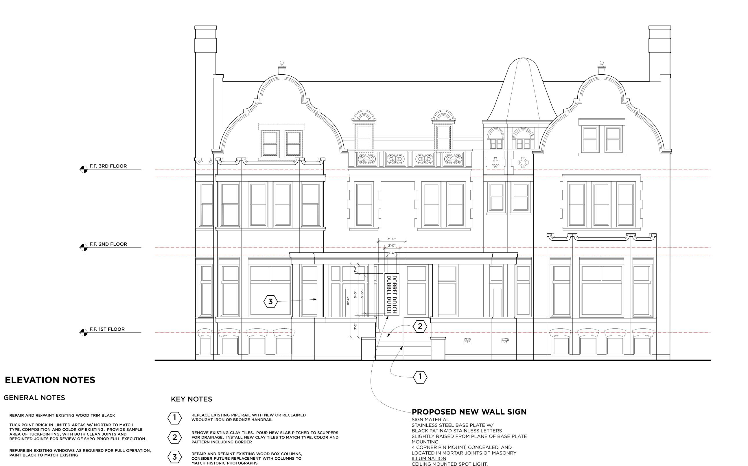
NEW CANOPY/HOOD SIGN 7" X 120" = 6.75 SF BRASS OR BRONZE LETTERS W/ GROUND PLACED SPOT UPLIGHTS CEILING MOUNTED SPOT LIGHT, SEE SP1.1 SITE PLAN FOR LOCATION
