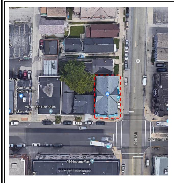
Aerial view of the property. Existing roof to be removed, damaged decking to be rebuilt, and new roof to be installed.
