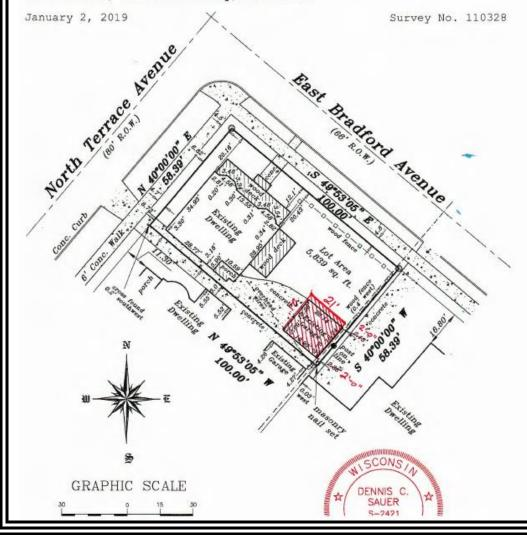
Survey including site plan indicating the location and dimensions of the new garage
