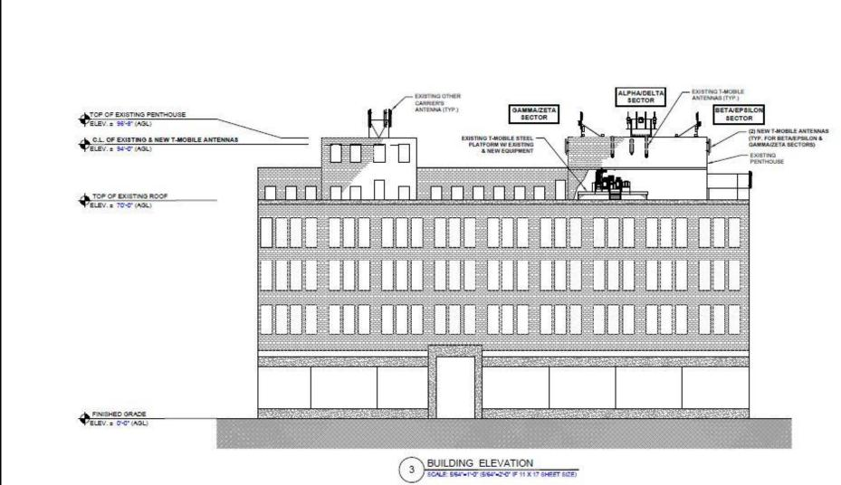
Elevation depicting current and proposed antenna configuration
