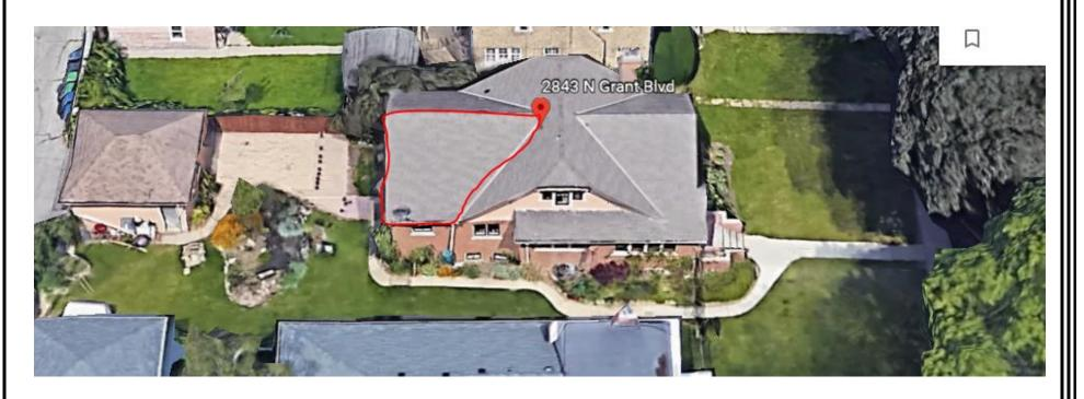
Solar panels are approved for installation only on the roof slope outlined in red. Required electrical equipment shall be installed on the rear (west) wall or the building interior.
