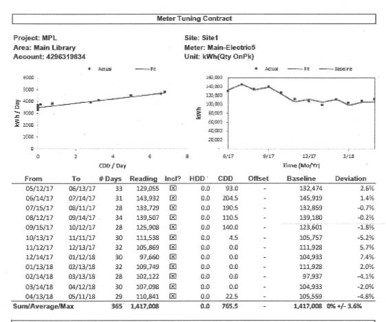
Main-Electric5 (Account # 4296319834): Tuning Period is 365 days from 5/12/2017 until 5/11/2018. Below is the equation used to calculate the Baseline values for the tuning period and all future periods: Baseline (kWh) = 3497.749 x #Days + 183.3175 x CDD
