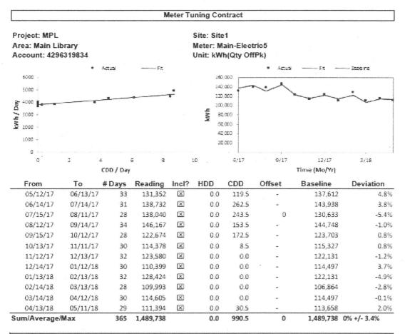
Main-Electric5 (Account # 4296319834): Tuning Period is 365 days from 5/12/2017 until 5/11/2018. Below is the equation used to calculate the Baseline values for the tuning period and all future periods:
