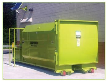
This major retailer is one of the first to adopt a "green" policy that included compaction equipment. This installation features a RJ-100 SC with a Solar Power Unit and Cushioned Ground Rollers.
