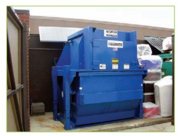
This solar powered power unit runs a Vert-I-Pack (VIP) at a national fast food restaurant. The solar energy is used to recharge two premium deep cycle batteries.
