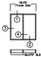
T-14000 I/O Inside Set / Outboard Flush Glaze Series Thermal Mock Up #1 - AAMA 1503
