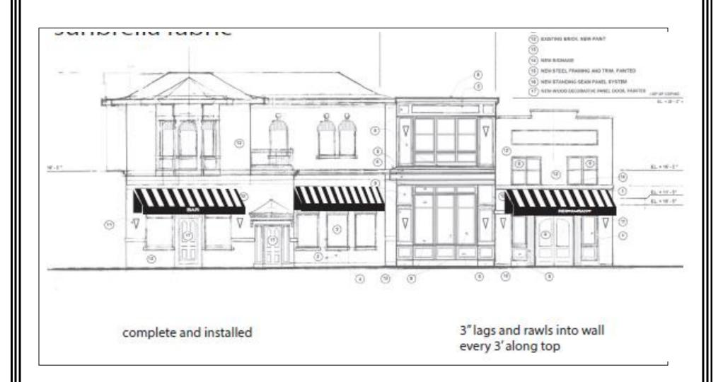
Awnings will measure 16'2", 13'5", and 15'10" in width. Lags will go into mortar joints not through face of the brick.
