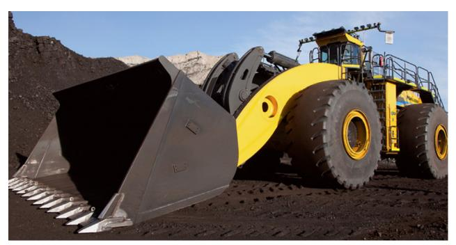
*P&H-brand L-2350* wheel loader features the standard bucket capacity of 40.52m3, about doubling that of KOMATSU-brand WA1200 wheel loader, the largest model conventionally offered by Komatsu.
