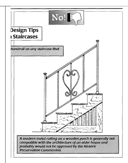
This design is acceptable WITHOUT CURLICURES for sidewalk/berm steps. This kind of railing may not be used on porch steps.
