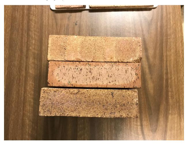
Top and boottom brick are original. Middle brick is approved for low-to-ground use on east and south elevations where new brick is needed. This would not be approved for highly visible elevations or significantly above grade.
