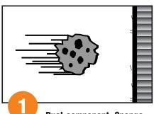
Dual-component, Sponge Media abrasives are propelled to the surface using an air-driven system
