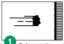
Single-component, conventional abrasives are propelled to the surface using an air-driven system
