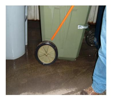
Another huge reoccurring problem is the cart bottoms freezing to the ground surfaces. This style cart has an extremely large flat surface area making it a prime candidate to adhere to the ground when placed in a wet environment and temperatures drop below freezing. It is very hard to break loose from frozen ground without cracking the plastic wheel housing causing wheel to fall off.
