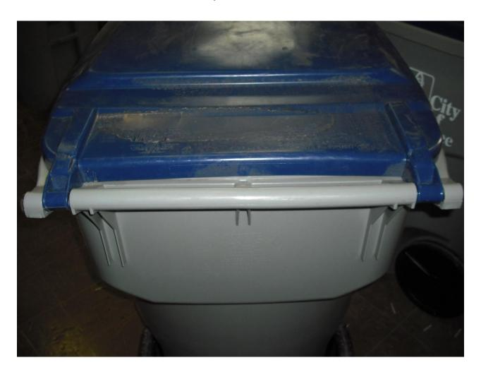
Repairing damaged carts: On the Zarne carts the handles and both upper and lower bars were replaceable in the field. On the other hand, when the grey carts get damaged, whether it's the handles, the hook-up point or the bottom bar, it's damaged beyond repair
