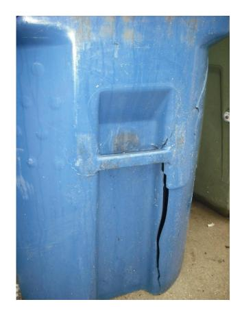
Both extremely low temperatures and excessive weight have a tendency to break the bottom plastic bar rendering the cart useless.
