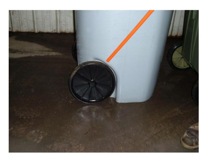
Note the fender overhang and lack of wheel clearance.
