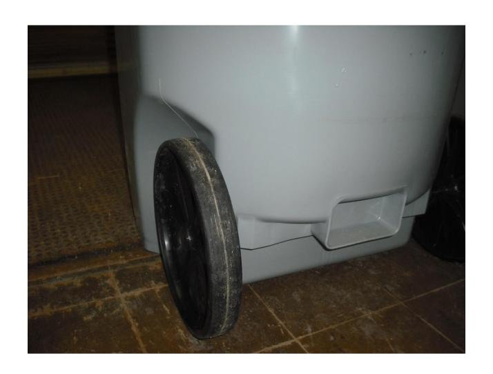
Zarne Cart: This cart had wide open wheels and was absent of all fender wells which eliminated almost all obstructions from jamming the wheels from turning. Moved unrestrictive in all types of weather.
