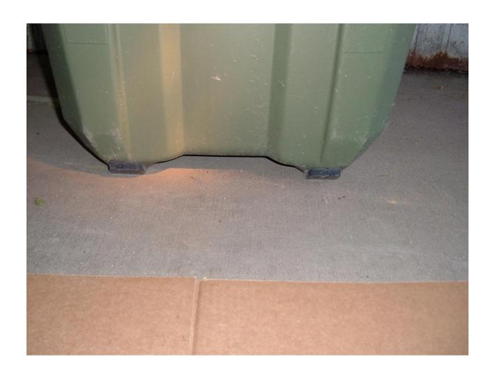
The picture on the left shows the Zarne cart has a clearance of four inches when tipped for transportation, whereas, the picture on the right shows the grey carts have a one and a half inch clearance.
