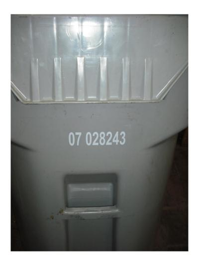
Lower bottom molded lock bar – snaps under a load, snaps in the cold and will snap if hooked up to an older style flipper. Limited area for bottom lock hook to grab.
