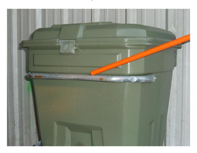
Note on the Zarne cart that the bar runs the entire front of the cart allowing the flipper to grab hold of the cart at any angle no matter if it's centered or off to the left or right.
