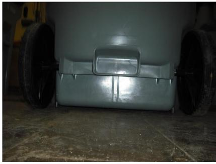
Note the upper hook up lip and the lower lock bar are constructed of all molded plastic. This plastic will snap away from the body during the dumping process when the cart is on the heavy side and both upper and lower sections will actually snap off and allow the cart to be thrown on cold days. Once either portion breaks away this cart is rendered useless.
