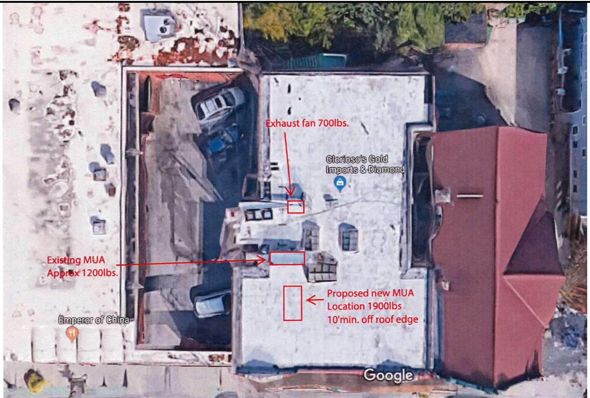
Rooftop equipment locations. All equipment must be painted, not visible from Brady Street, or both.
