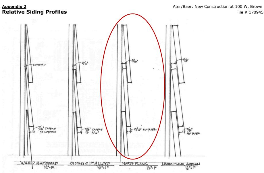
The figure above shows the relative thicknesses (actual, not advertised) of the following siding products (left to right): Eastern White Pine from Ward Clapboard Mill (Vermont); Cedar siding being used on post-fire rehab property at the corner of 1<sup>st</sup> and Lloyd in Brewers Hill (measurements taken on the building site); HardiePlank Smooth Lap Siding ("regular" HardiePlank); HardiePlank Artisan Lap Siding. **We propose to use HardiePlank Smooth Lap Siding 5/16" siding (circled above).**
