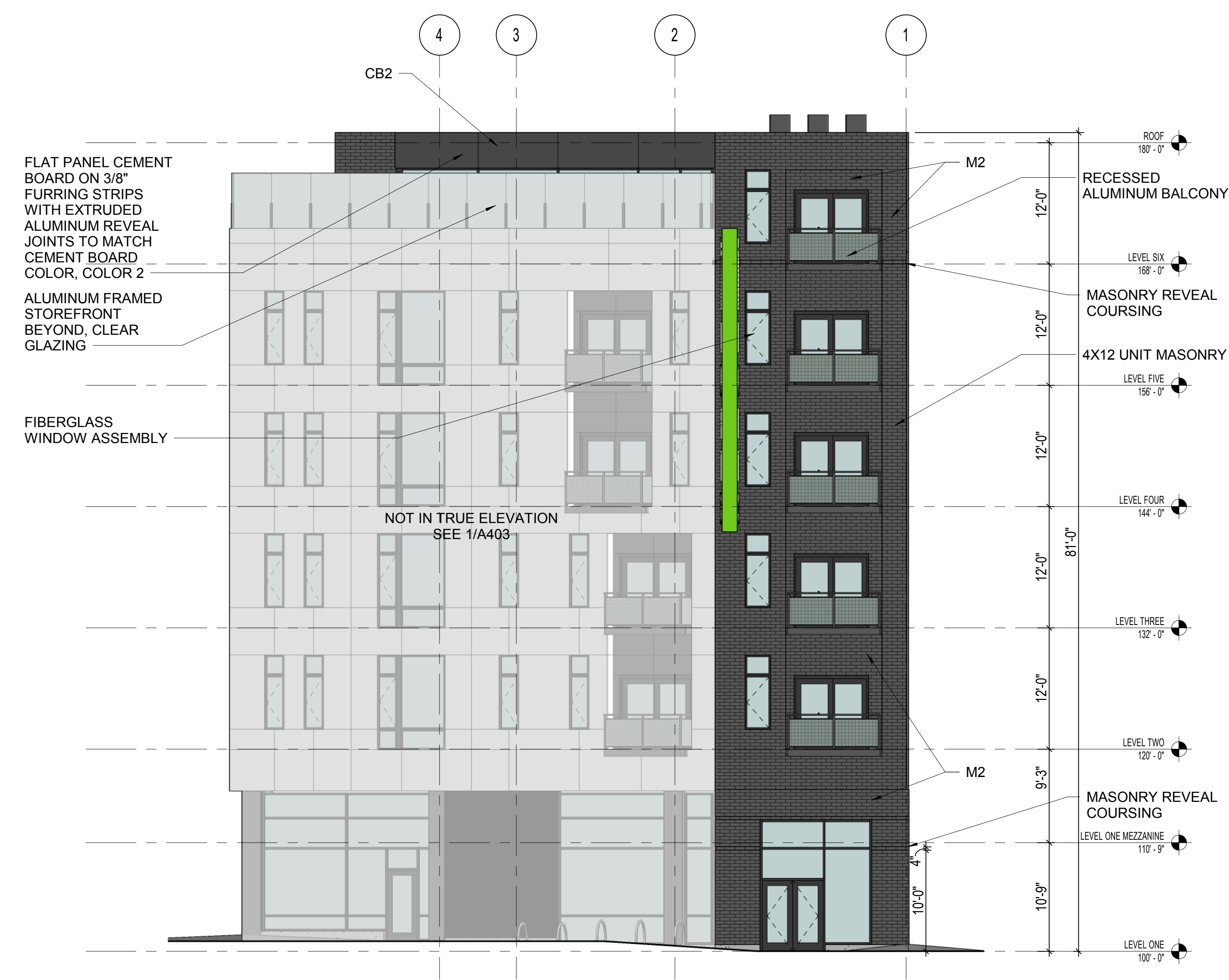
2 SOUTH ELEVATION - FLAT SCALE: 1/8" = 1'-0"
