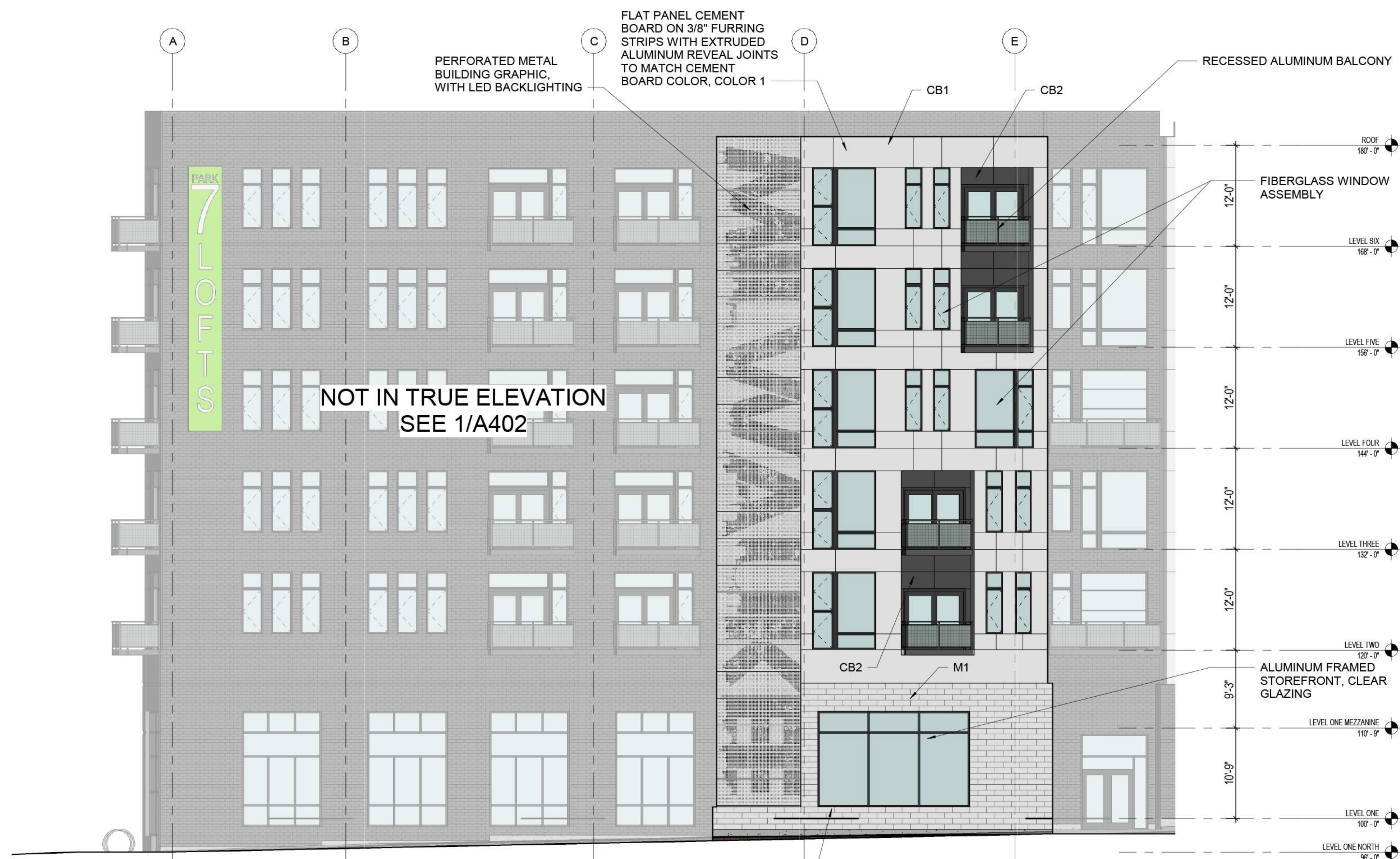
1 WEST ELEVATION - ANGLED (NORTH HALF) SCALE: 1/8" = 1'-0"
