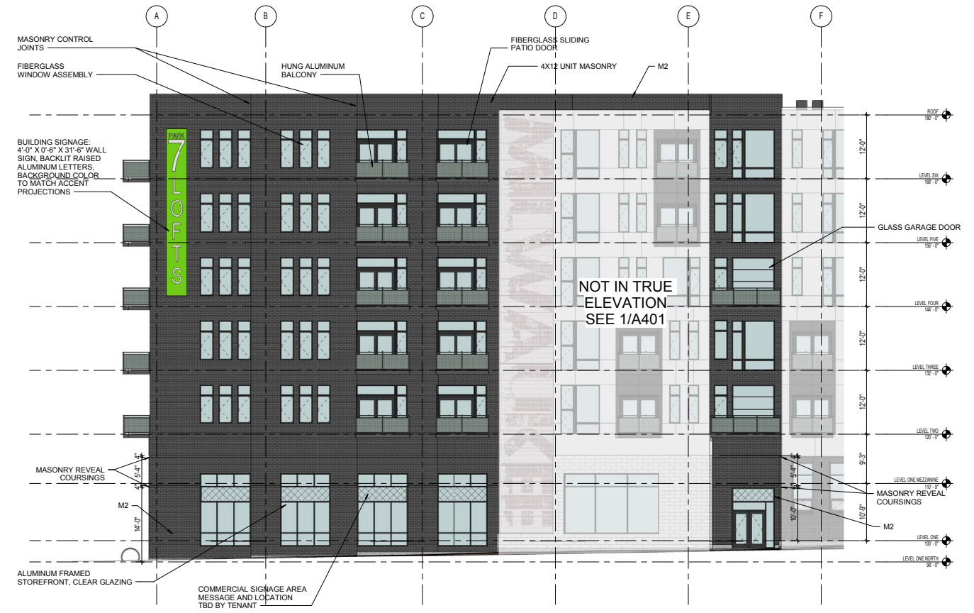
1 WEST ELEVATION - FLAT (NORTH HALF) SCALE: 1/8" = 1'-0"
