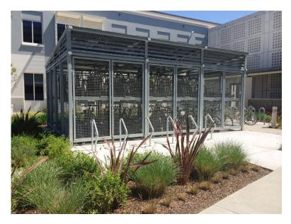
Allows unique, different style racking systems for expanded amount of bicycle parking, however REQUIRES that the minimum number of spaces required by code are at ground level.
