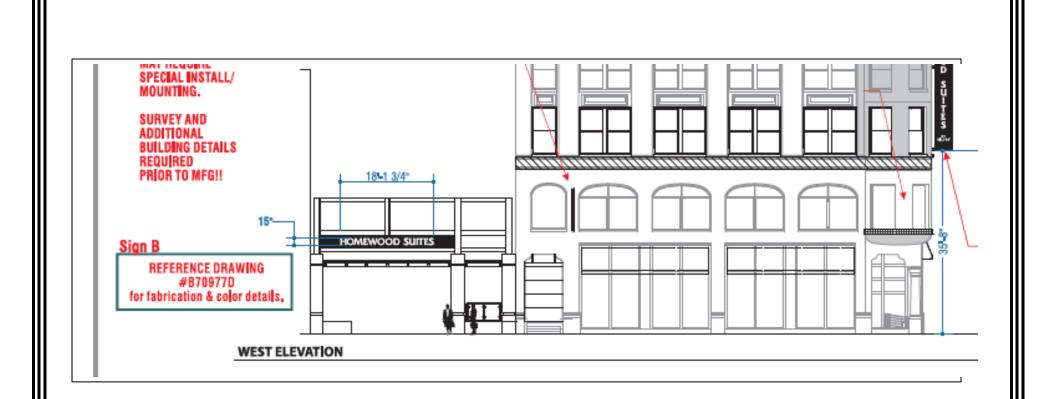
Sign B consists of a 26' long by 1'3" tall by 5" thick aluminum illuminated wall sign with push through copy. It will be installed at the entrance to the drive up area along North Water Street.
