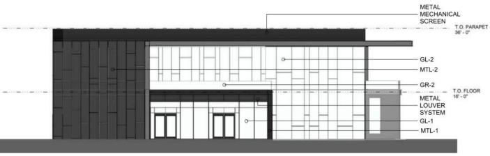
BUILDING B - NORTH (PEDESTRIAN CONNECTOR) ELEVATION 1" = 10'
