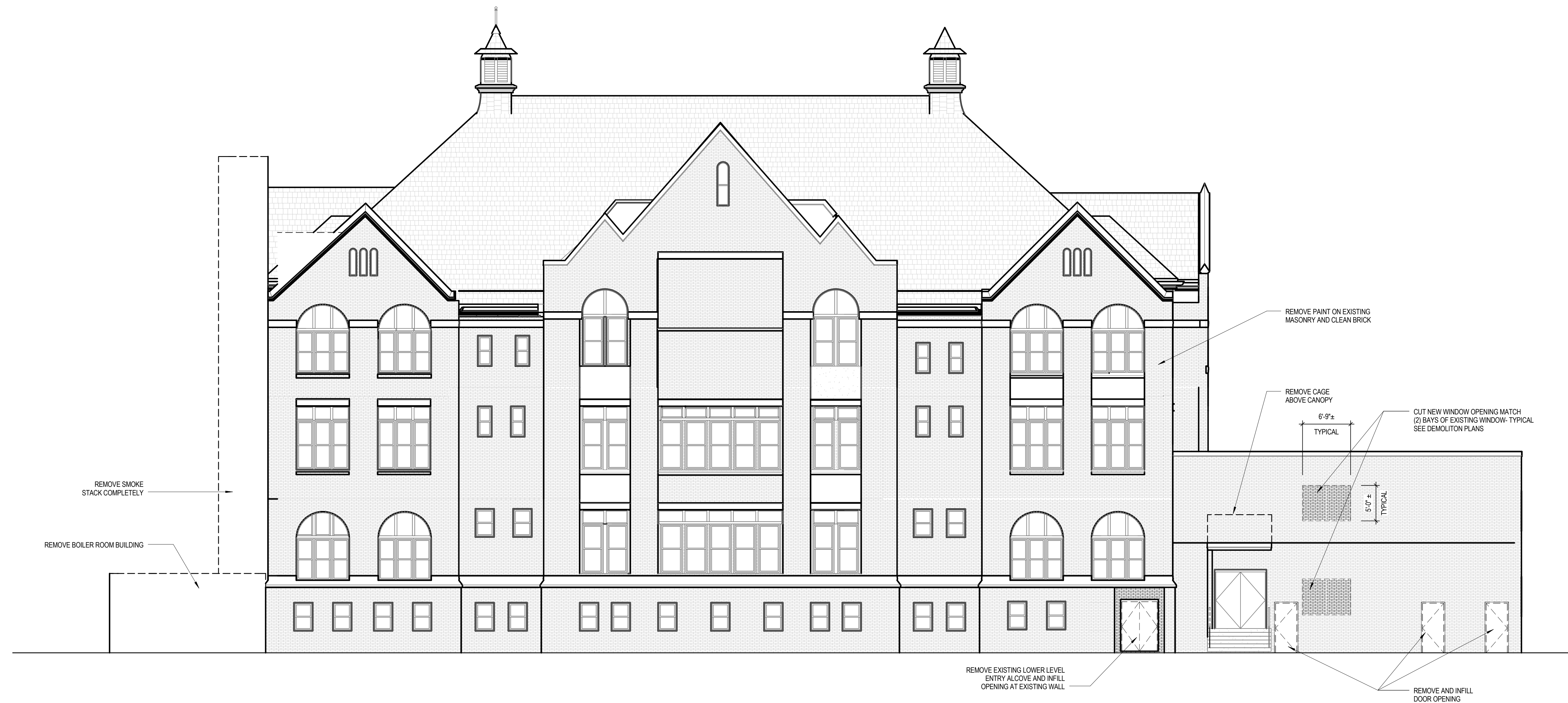
1 WEST DEMOLITION ELEVATION SCALE: 1/8" = 1'-0"
