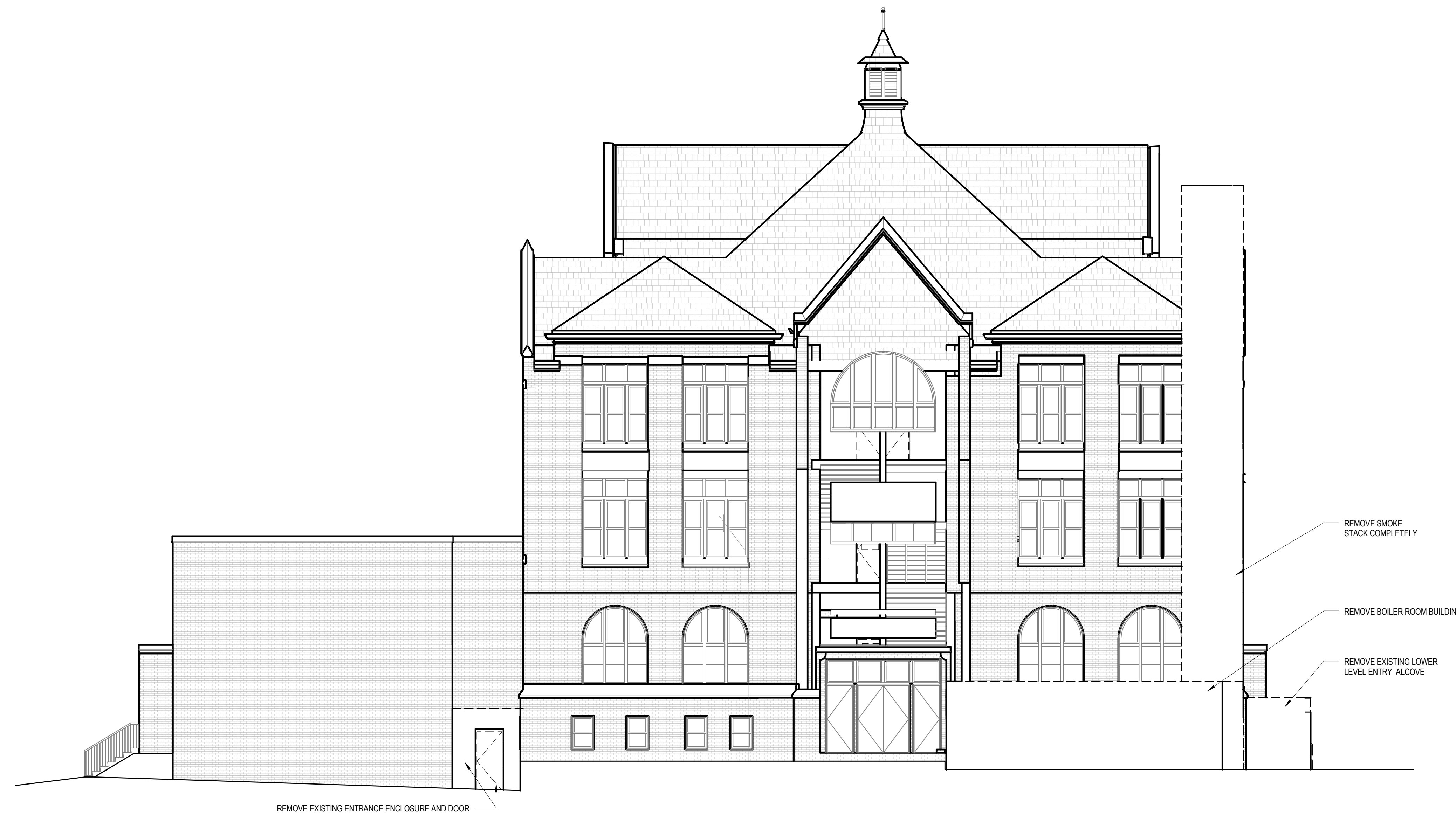
2 NORTH DEMOLITION ELEVATION SCALE: 1/8" = 1'-0"
