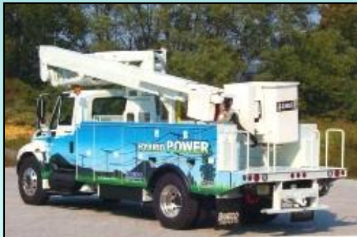
Hybrid Aerial Bucket Truck (On Order) Operates on Batteries Reduces noise, emissions and Fuel Payback = 6 years
