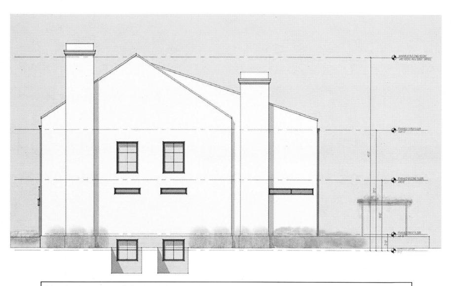
North elevation of the new house. Vents will be located for the most part to the rear of the front chimney and that will help to minimize them from the front right of way.
