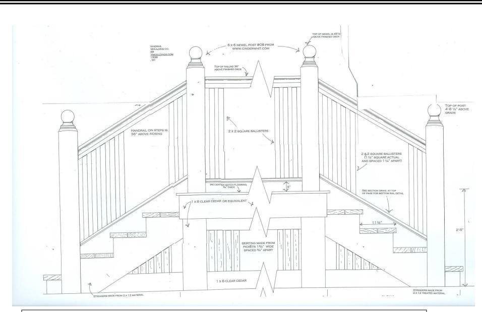
Top rails will have "breadloaf" or other graspable shape. Bottom rails will be tapered to shed water. Balusters will be 2 x 2 wood and spaced 1-1/4 inches apart.
