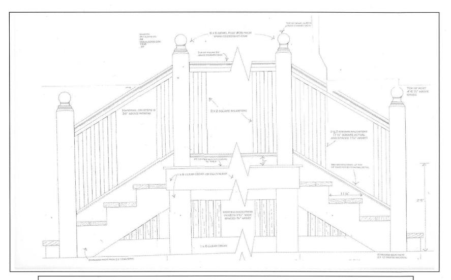
This is acceptable railing design but newels should be built according to design on next page.
