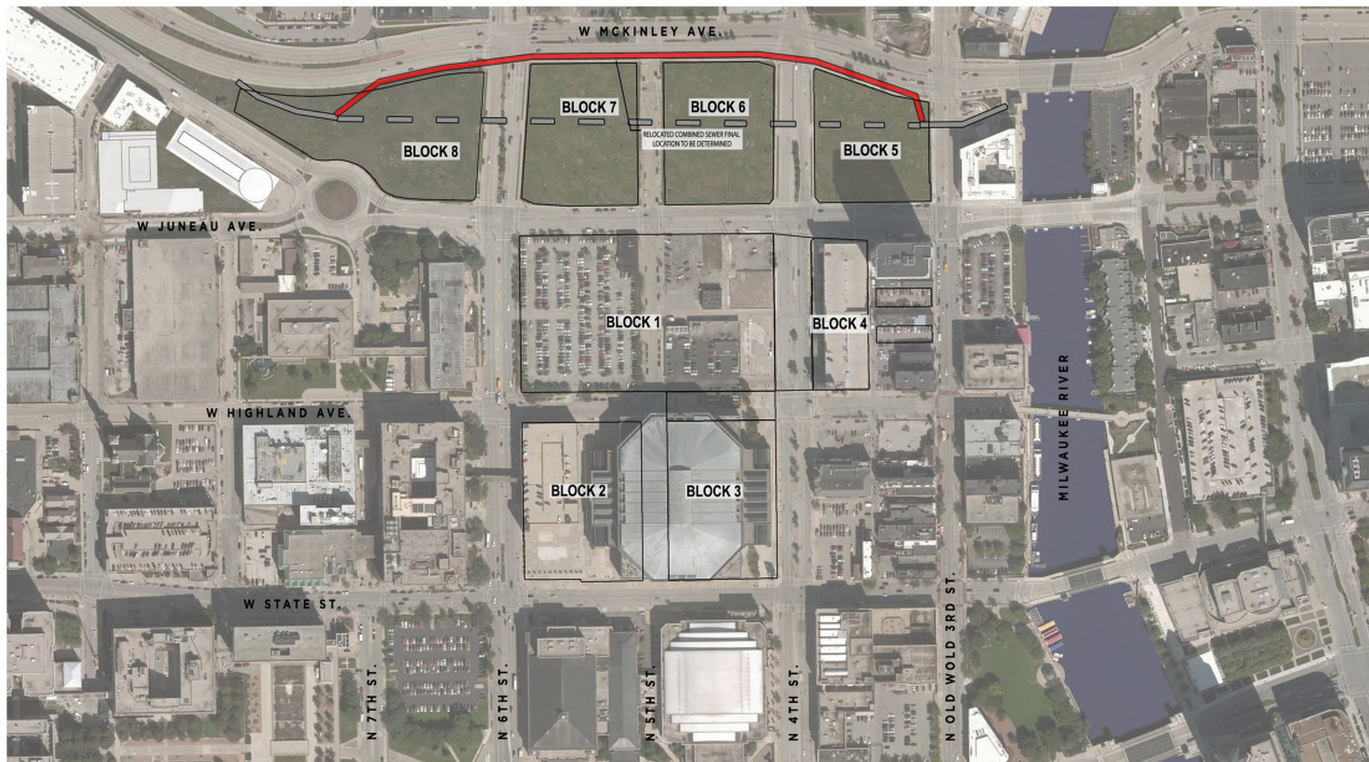
CONSTRUCTION SEQUENCE 1A: RELOCATE EXISTING COMBINED SEWER ALONG MCKINLEY AVENUE.
