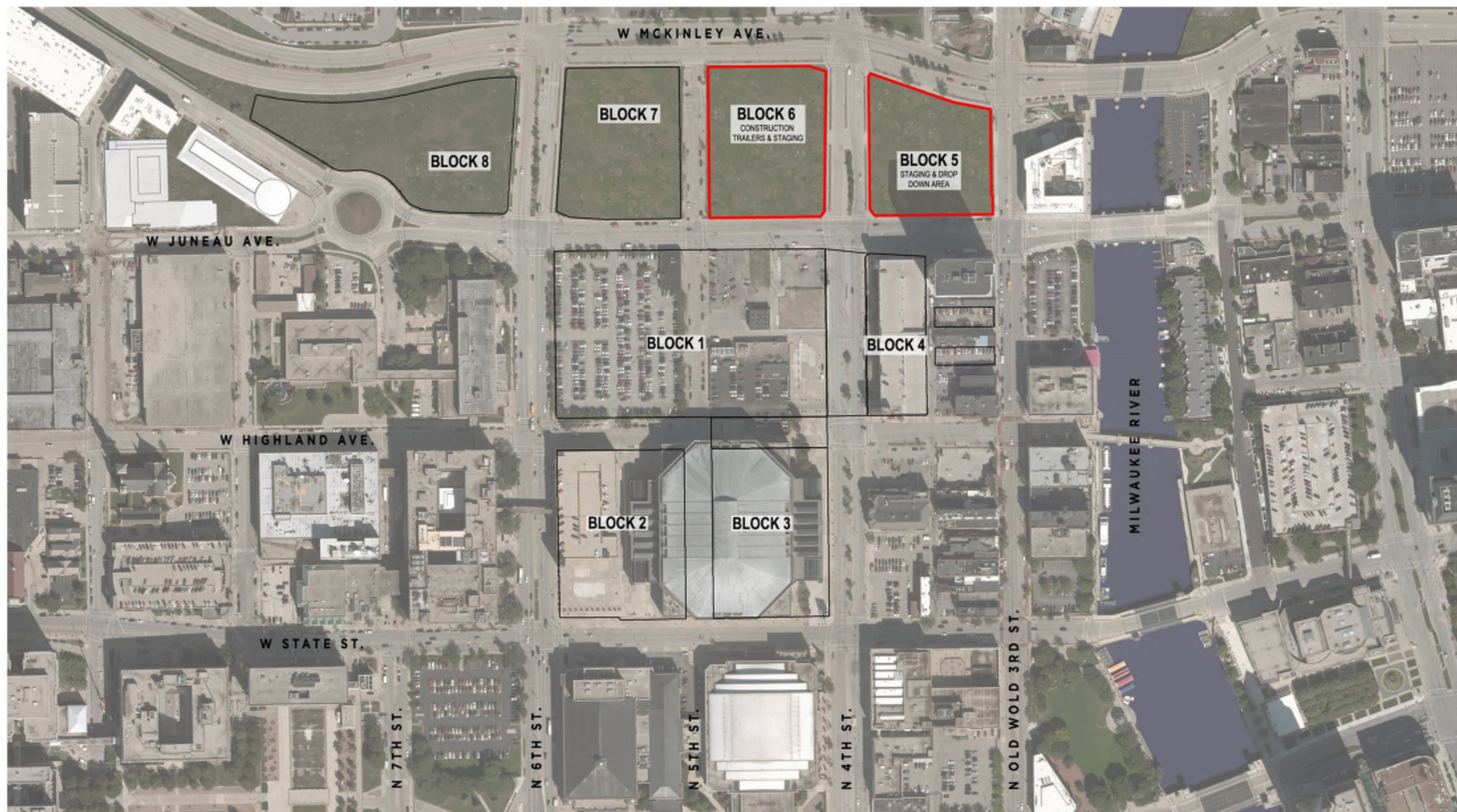
CONSTRUCTION SEQUENCE 1B: BLOCK 5 & 6 TO BE FENCED FOR CONSTRUCTION TRAILERS & STAGING DROP DOWN AREAS.
