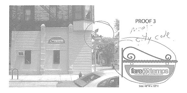
West building elevation with 82"W x 30"H Dibond wall sign and 48"W x 18"H double sided Dibond hanging Scroll bracket sign
