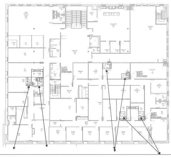
The HVAC units will be installed at the locations indicated but at the rooftop. They will not be visible or only minimally visible from the right of way.
