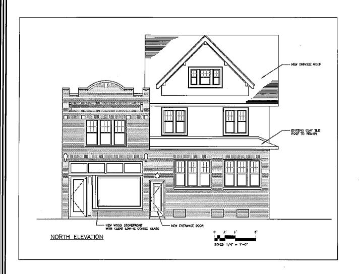
New asphalt shingle roof to be installed. Tile pent roof to remain.
