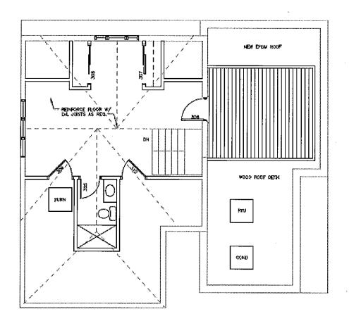
New wood deck on rooftop will be screened by parapet wall.
