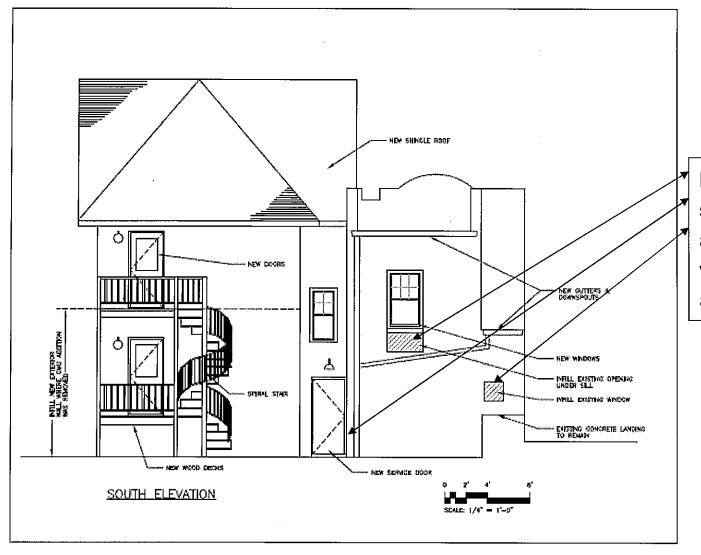
Note: new service door, infill at opening below window and infill at small window
