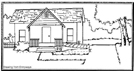
Many feet can be shaved from the required length of an incline if it starts on ground that is nearly the same elevation as the entrance. Here, the driveway is sloped to provide some rise on a flat lot.
