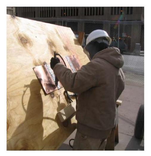
Mechanic Soldering Test
