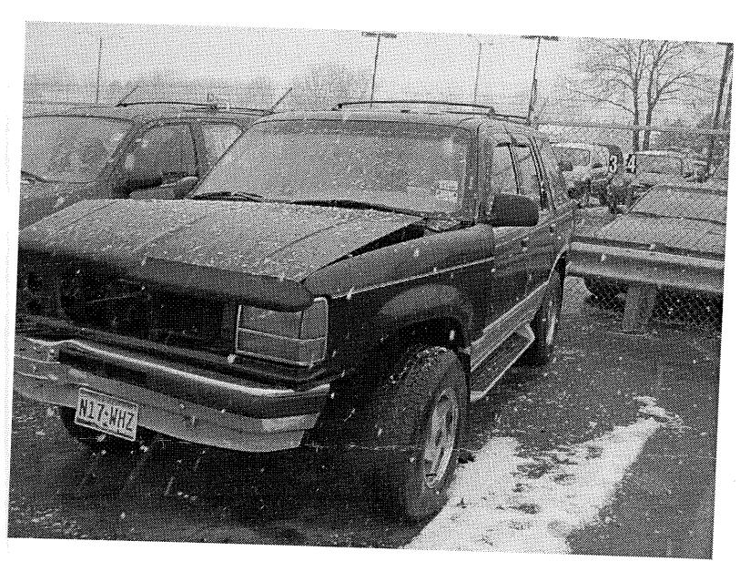
This picture shows how there was no impact damage to my drivers side, which would have been hit if I were at fault and pulled out. No damage other than the frame being pulled over by the gas truck clipping my vehicle.
