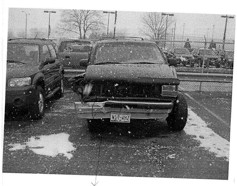
This shows the impact damage 2/3 of the way across the front of my vehicle. The passenger side fender ripped outwards shows my vehicle also being clipped and pulled away from the body.
