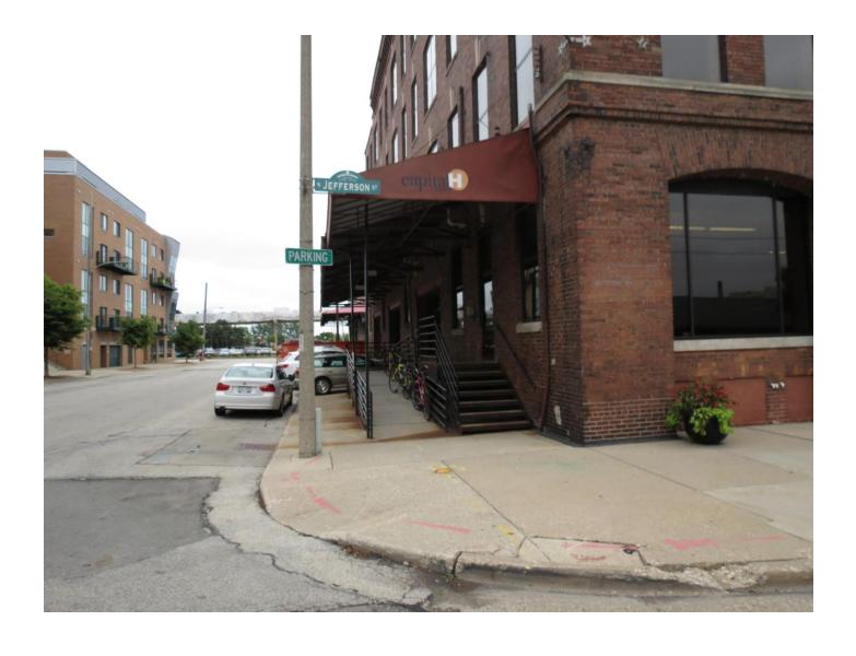
CCF 090496 120 North Jefferson Street 9-11-2014 Looking east at the south sidewalk area of East Corcoran Place. Note that there is a 5-foot clearance between the light pole and the ADA ramp structure.
