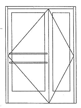
Drawings of new doors with original hardware reinstalled. The door on the right with a side-lite will be
