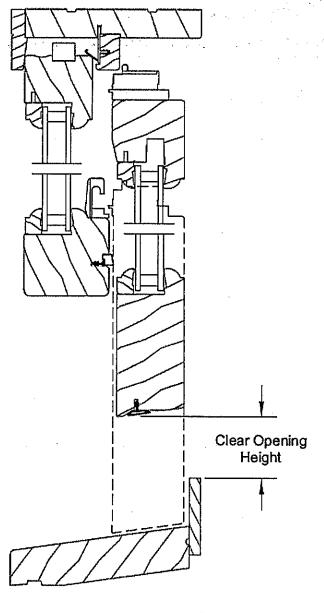
Section of new wood windows for replacement on sides and back and attic windows in front. Any muntins in replacement units must match exactly the profile and size of the originals and must be permanently fixed to the window (no removable grills.)
