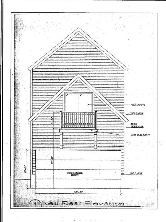
Rear elevation showing new garage door and balcony.
