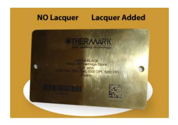
MATERIAL: 260 Brass - 24 Gauge (.0250" thick), brushed and polished finish. Brass is beautiful but if you're looking for durability, Stainless Steel is the best. Brass will tarnish and scratches easily. Add lacquer for outdoor protection.
