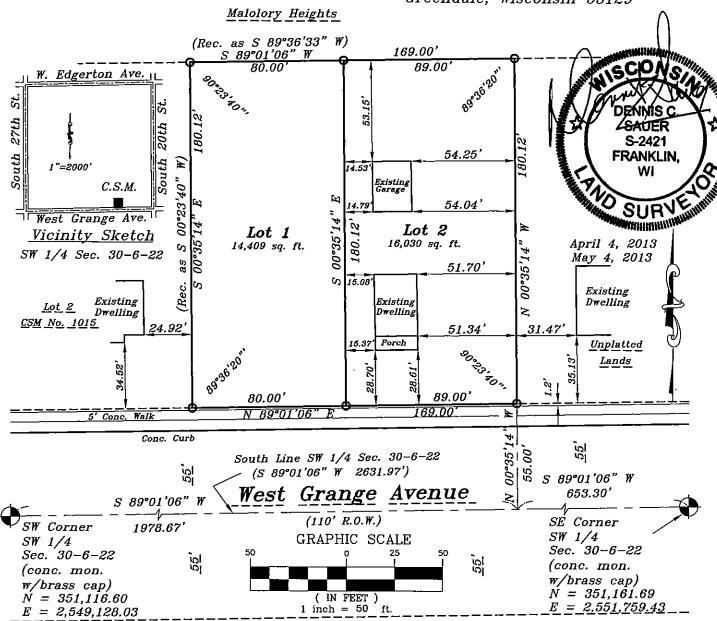
Map bearings refer to Grid North of the Wisconsin State Plane Co-ordinate System, South Zone, with the South line of the SW 1/4 of Section 30, T6N, R22E having an assumed bearing of S 89°01'06" W. December 2011 Datum
