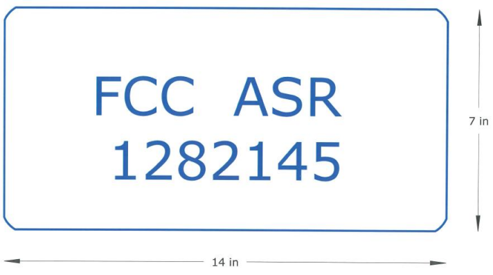
FCC REQUIRED SIGN TO POST ON THE TOWER
