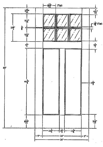
Elevation drawing of new wood door to replace existing metal door
