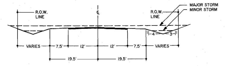
**ROADWAY WITH CURB AND GUTTER**
