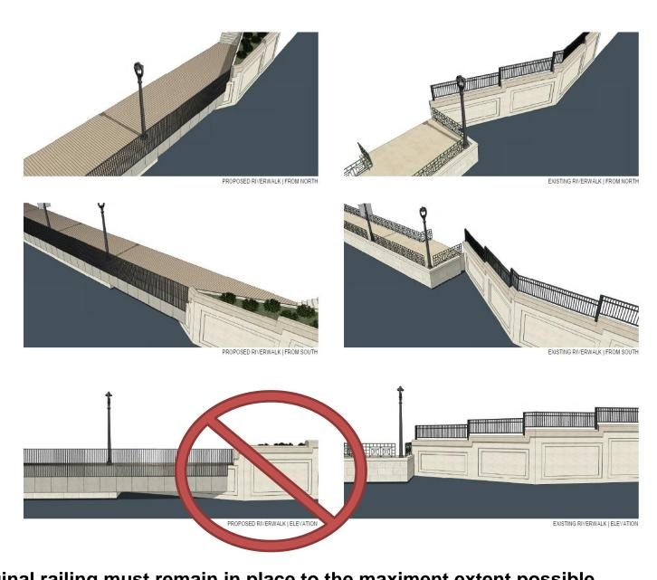
Original railing must remain in place to the maximent extent possible. Remove railing only from the tier that is being shortened.
