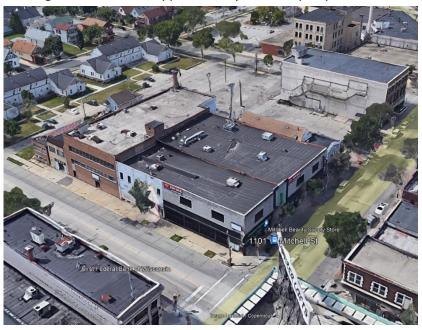
and vacant office space on the 2<sup>nd</sup> floor. A school was constructed in the basement which is vacant. An addition was built in 1949 to the south of the original building and was constructed with steel and concrete framing. The 1949 addition is approximately 8,700 sq. ft. per floor and has two mezzanine levels located between the 1st and 2nd floors, approximately 2,800 sq. ft. The western half of the 2<sup>nd</sup> floor is constructed with concrete slabs and was used for a vault area to
