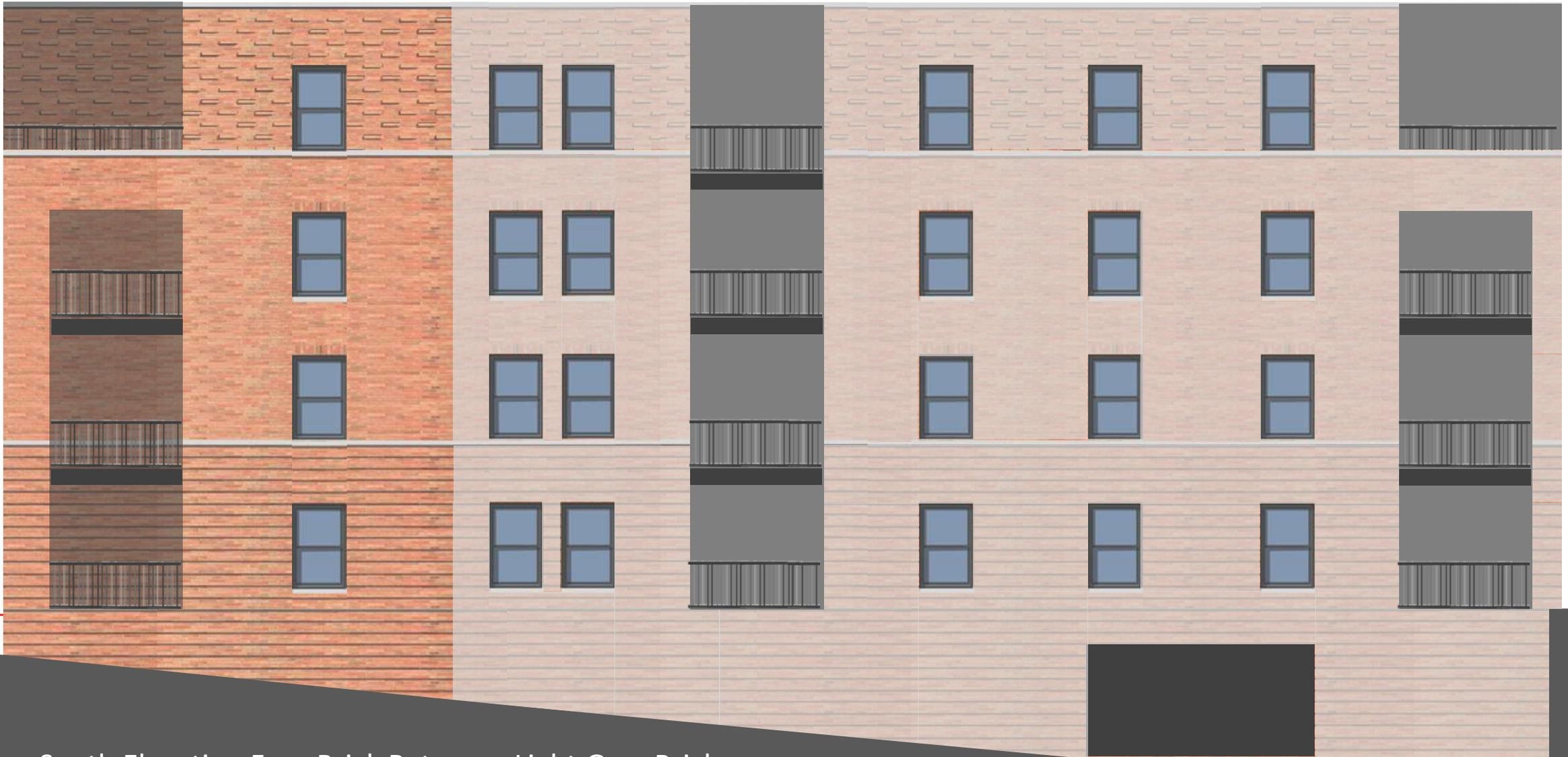
South Elevation Face Brick Return w Light Grey Brick
