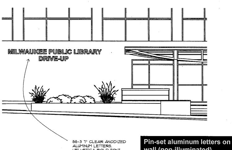
HELVETICA BOLD FONT SIMILAR TO CAST METAL LETTERS BY GEMINI INCORPORATED OR ARCHITECT APPROVED EQUAL. STUD INSTALLATION NO MORE THAN 1/2" SPACING FROM WALL SIGN HAS NO ILLUMINATION.
