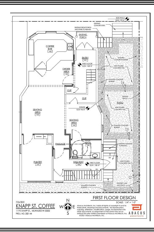
The poured concrete slab with decorative border will be located in the east side yard and serve to handle drainage, help with accessibility to two entrances and serve as outdoor space for the café.
