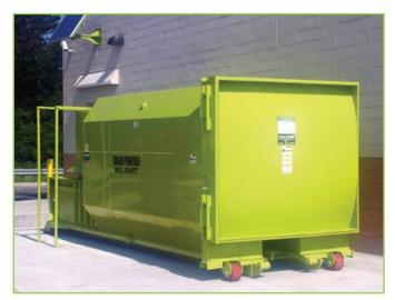
This major retailer is one of the first to adopt a "green" policy that included compaction equipment. This installation features a RJ-100 SC with a Solar Power Unit and Cushioned Ground Rollers.
