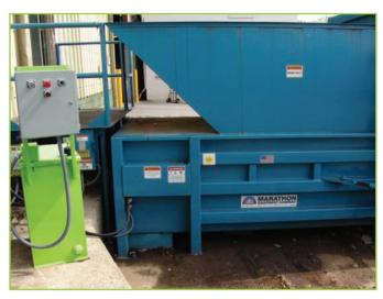
This GreenBuilt® 5 HP high efficiency submerged power unit runs a RAMJET 3 cubic yard TANK® located at a manufacturing facility. It provides the same speed and performance as its 10 HP predecessor.
